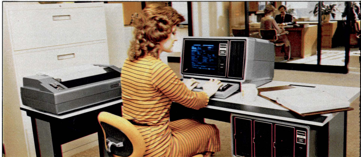
This TRS-80 system includes: 64K Model II (26-4002), 3-drive external disk system (26-4162) for a total of 1,874,000 free bytes of disk storage, Line Printer V (26-1165), Printer Cable (26-4401), System Desk (26-4301), and Printer Stand (26-4302).
